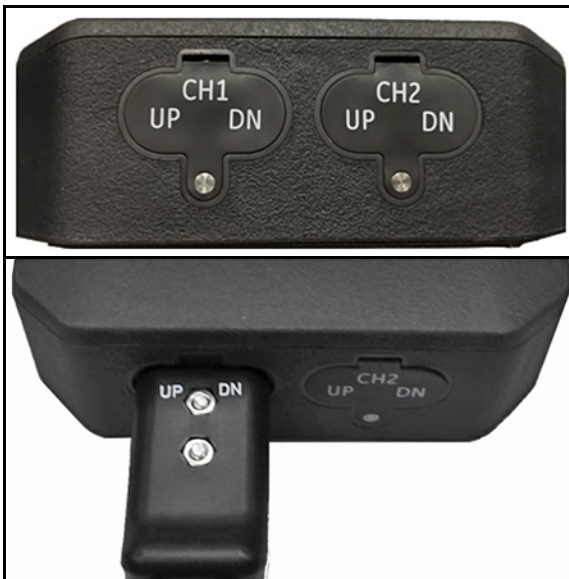
Figure 45: Transducer Connections (Bottom)
