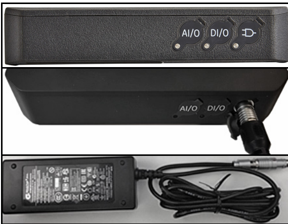
Figure 44: Transmitter Power Connection (Right Side)
