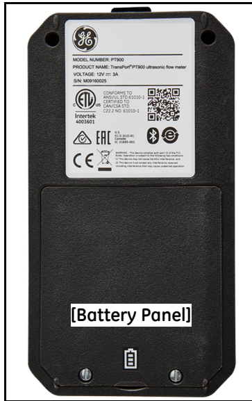
Figure 50: Battery Panel Location
