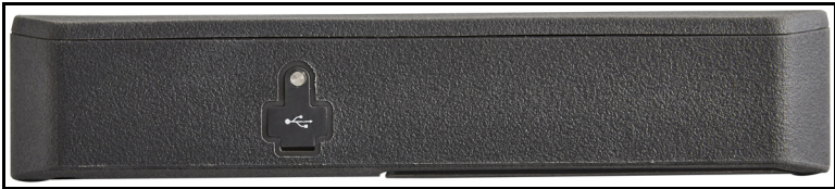
Figure 48: Transmitter USB Connector (Left Side)
