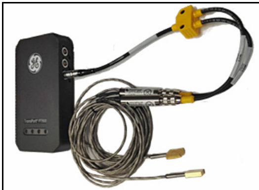
Figure 47: Energy Cable Connection (Right Side)
