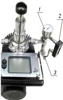
ILLUSTRATION 15: Gas flow and gas pressure control system
