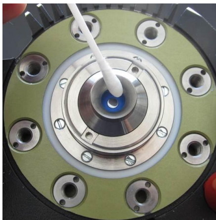
Illustration 16: Cleaning the mirror
