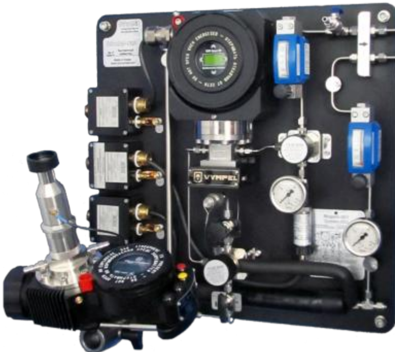
Illustration XI: “SGA 003” equipped with a “Hygrovision mini” as the reference analyzer
